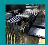
Intelligent feeders in all common sizes Component spectrum from 0402 to 18x20 mm
